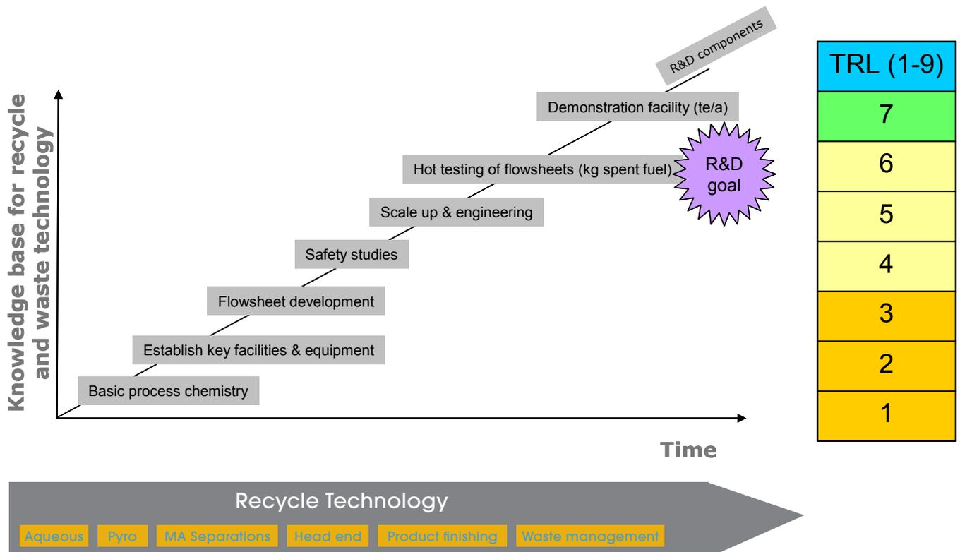
Figure 4: Development ladder for advanced reprocessing technologies; showing links with Technology Readiness Levels and a realistic target date for first hot tests of new (aqueous) separation processes in a UK facility (5-10 year goal)
