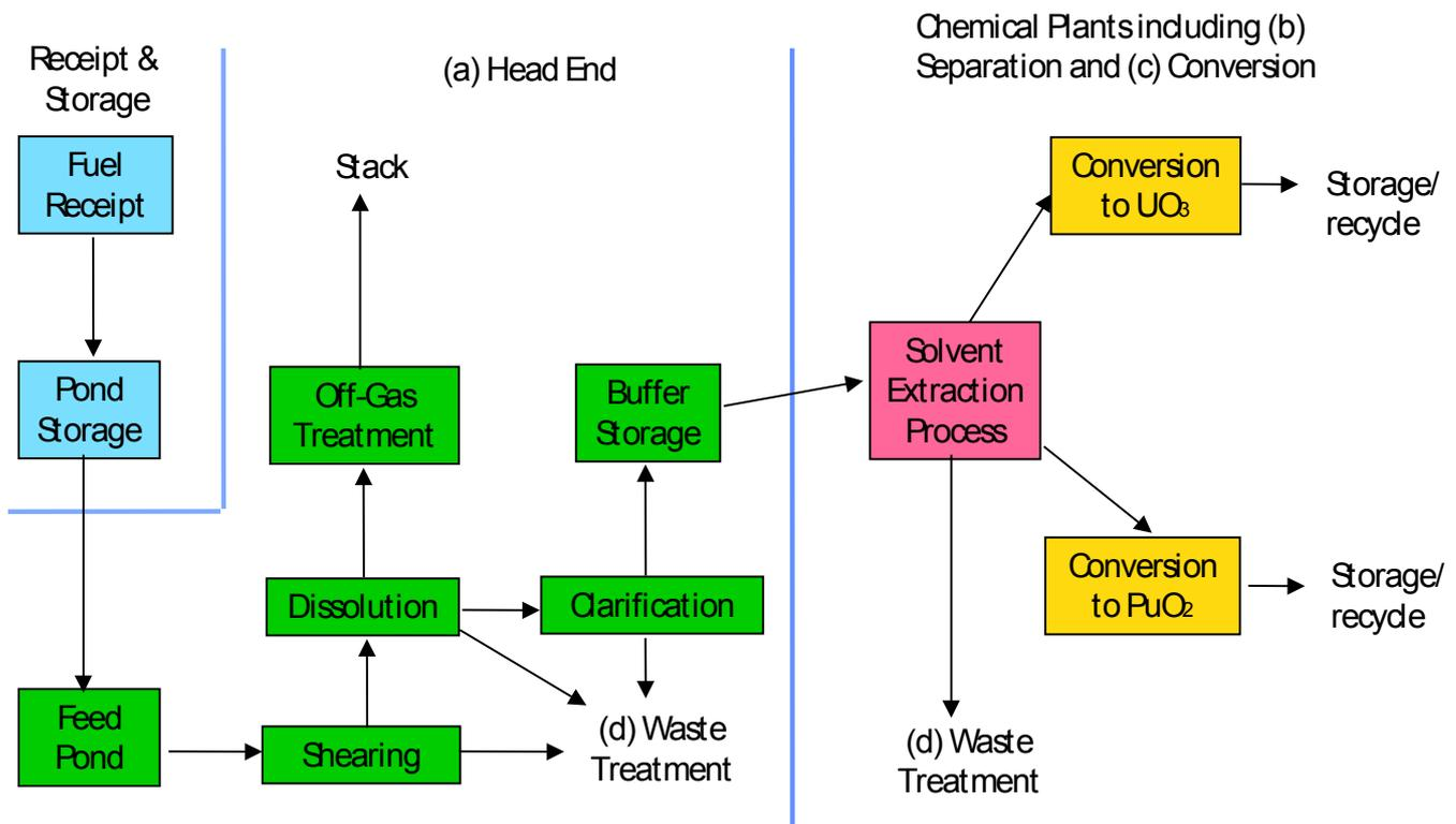
Figure 5: Schematic representation of a typical configuration for an oxide fuel reprocessing plant using the conventional PUREX process, indicating (a) Head End, (b) Chemical Separation, (c) Product Conversion or Finishing and (d) Waste and Effluent Management.
