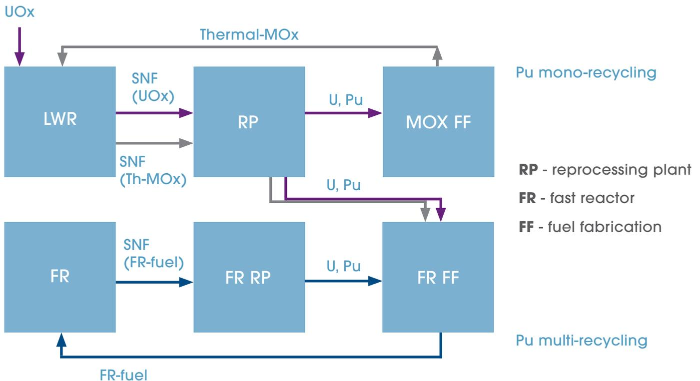
Figure 2: Schematic illustration of plutonium mono- and multi- recycling scenarios
